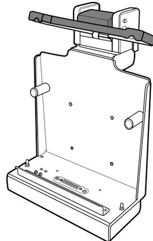
To release the upper latch, push the latch backward. The upper latch plate is automatically released.
